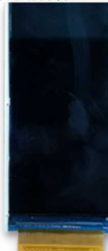
2.99" IPS TFT LCD, SPI 268X800 Pixels
