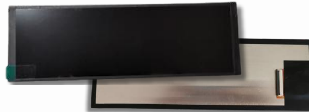
7.84" IPS TFT LCD, MIPI/LVDS, Touch option High-brightness, 400×1280 Pixels
