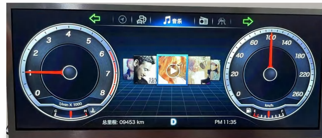
12.3" IPS TFT LCD, LVDS 1920×720 Pixels
