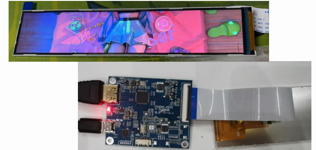
7.1" IPS TFT LCD, MIPI/HDMI option 280×1424 Pixels
