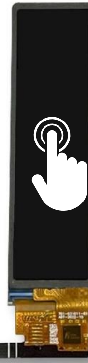
3.18" IPS Touch LCD, MIPI 288X960 Pixels
